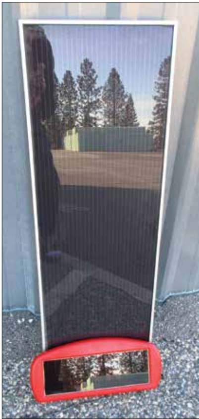
A tall 25-watt Harbor Freight solar cell and a short 1.5-watt (red) Harbor Freight Solar Cell. The reflections on the surface of the cells are the hangars across the taxiway.
