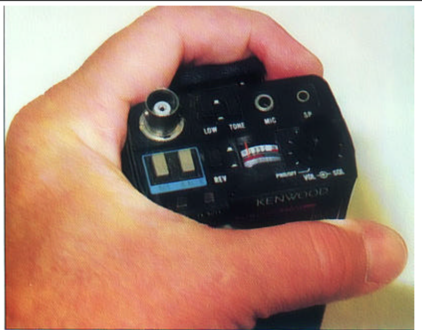
Handheld transceiver manufacturers such as Kenwood use this connector series.
