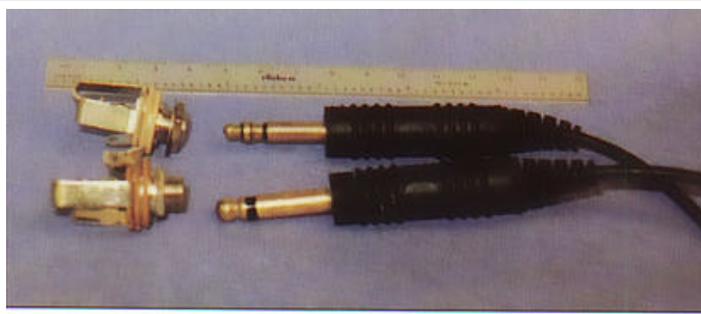
Mil-spec versions of the 1920s-technology mic plugs and jacks are brass that corrodes, causing intermittent connections.
