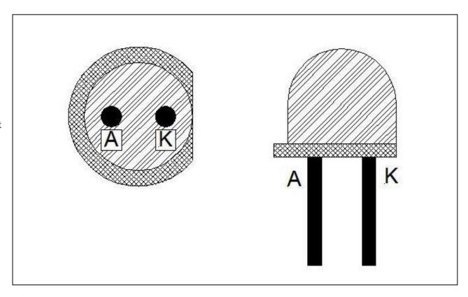
Note that the "skirt" (bottom of the LED) has a FLAT on one side of it. This positively identifies the cathode end of the LED. As shipped from the factory, the cathode wire lead is shorter, but you cannot guarantee that somebody didn't clip the anode lead from the LED and put it back into the stock bin.
