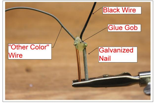
the other side of the electrodes and allow the glue to thoroughly dry.
