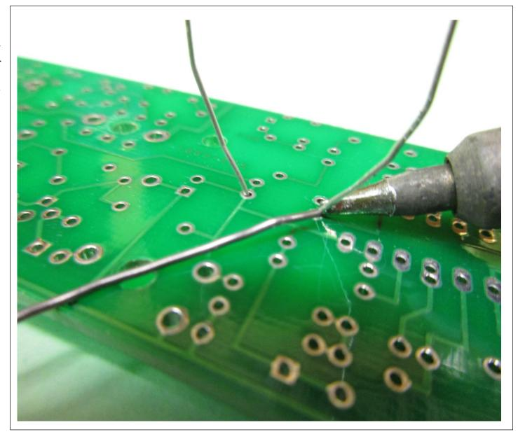
k. A nice round joint of solder is inspected, the excess lead cut off, and you move on to the next joint.
