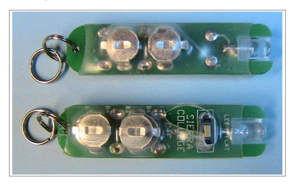
The LED flashlight is what we call a "complete circuit". It has the four basic elements found in all electronic circuits -- **Source, Load, Conductors, Control.**
