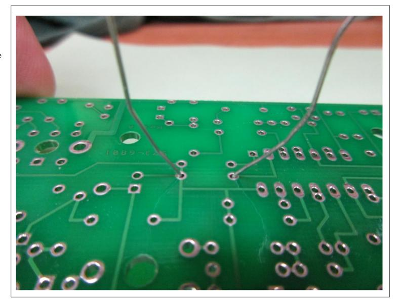
j. The hot soldering iron tip is brought in from one side of the joint, the solder is brought in from the other, and THE JOINT IS HEATED so that the solder melts onto the joint, not the iron.
