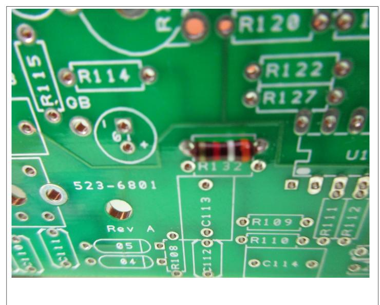
i. Component leads go through the holes in the board and are bent out at a 45° angle to keep the part from falling out of the board.
