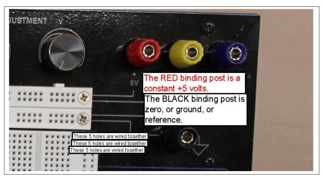
d. Take your multimeter and prove to yourself that the voltage between the red binding post and the black binding post is between 4.9 and 5.1 volts.
