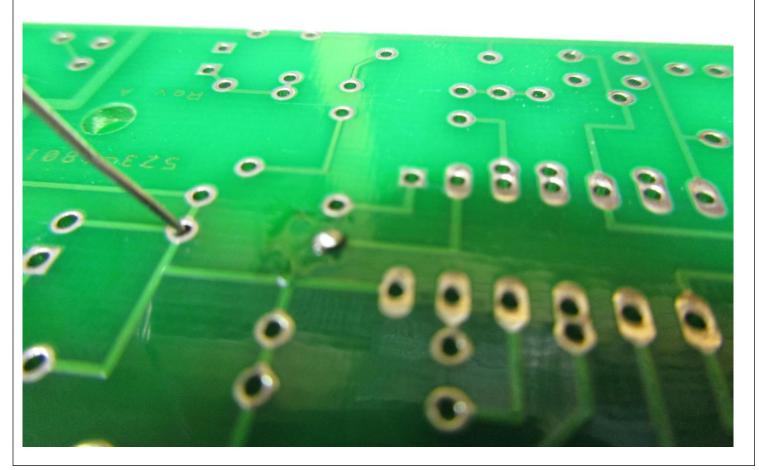
1. OOPS, you put the wrong part into the holes. Not to worry. Desoldering braid to the rescue. Desoldering braid is just copper braid soaked in flux. The solder on the joint is MUCH happier to wick up into the braid than stay on the joint.
