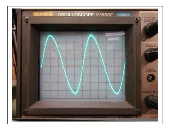
3. We can also measure the voltage of this sine wave. Note that the vertical "y" axis is calibrated as 2 volts per division, so from the center zero volts line we go UP 4 divisions (8 volts) and DOWN 4 divisions (-8 volts) or a "peak to peak" voltage of 16 volts.
