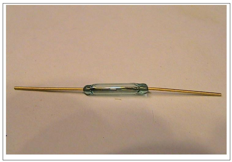
i. The switch is "normally open 'NO" Move the magnet around the switch at various angles and distances. Is there an optimum orientation where you can cause the switch to "close" or "make" at the longest distance?
