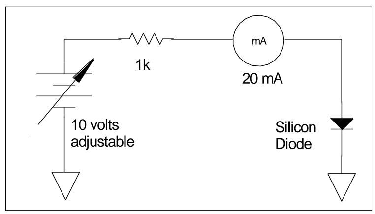
1. Equipment: Trainer, Two (2) digital multimeters. Use one of the digital multimeters to set 10.0 volts at the yellow (positive) binding post with respect to the black (common, ground, negative) binding post. Take a  $1k\Omega$  (brown-black-red-gold) resistor, the second digital multimeter set on the 20 mA full scale position, and a silicon switching diode (1N4148, 1N914, etc.); connect them as shown in this diagram.
