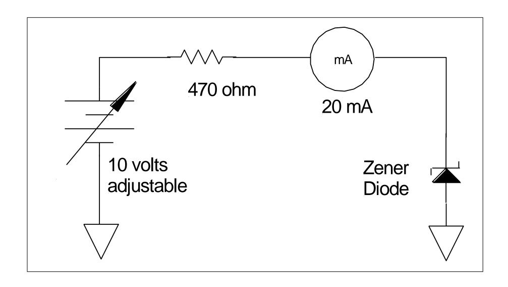
. Repeat steps 5 and 7 for a 5 volt Zener diode connected in REVERSE bias as shown on this diagram. (470 ohms – yellow, violet, brown, gold). Measure in steps of 2 mA per step. Record the results on the graph paper supplied on page 7 of this lab.
