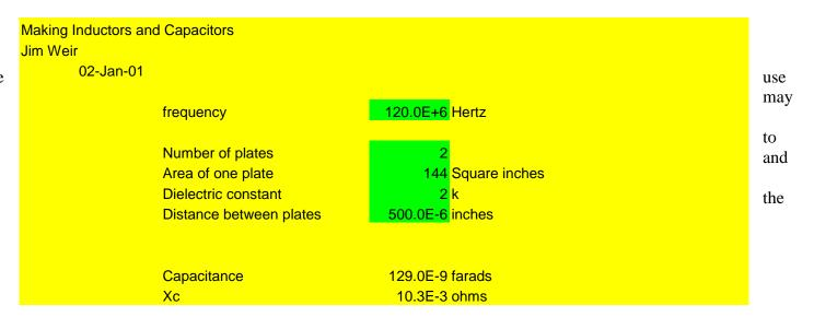
Well, now I know how to make capacitors and what their values will be, but so what? What is the use of a capacitor in an electronic circuit?
