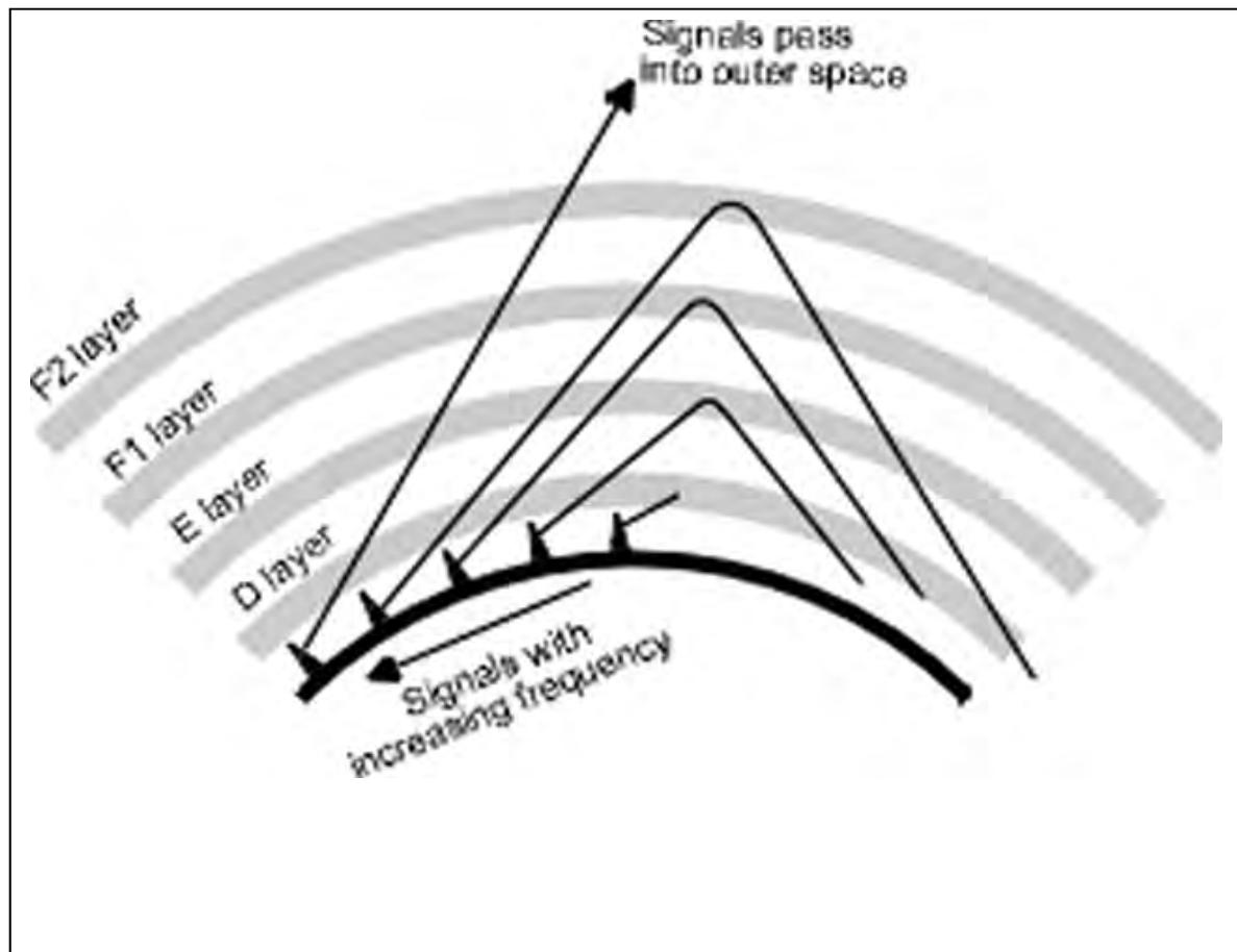
Signals above 30 MHz. generally do not bounce off of any layer, but instead just keep on going out into space. However, during periods of extremely active solar flares (the "sunspot" cycle) signals up to 150 MHz. can be reflected from the F layers. The next sunspot cycle peak is due to occur in late 2023 or early 2024 and is supposed to be the strongest series of flares since the monster year of 1985.
