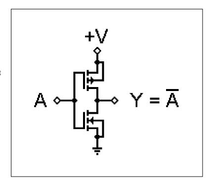
We generally have what is called a "truth table" in the data sheet for the device in question. The truth table tells us what will happen at the output for any combination of inputs. The truth table for this simple device looks something like this:
