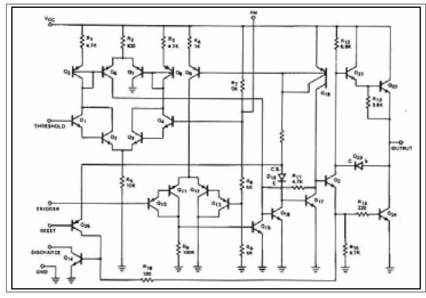
We like to say that there are "linear" integrated circuits and "digital" integrated circuits, but the 555 is really neither. It is analog in that it uses the charge-discharge of a capacitor to make itself work, but it is digital in that it outputs a pulse waveform that is either high or low.
