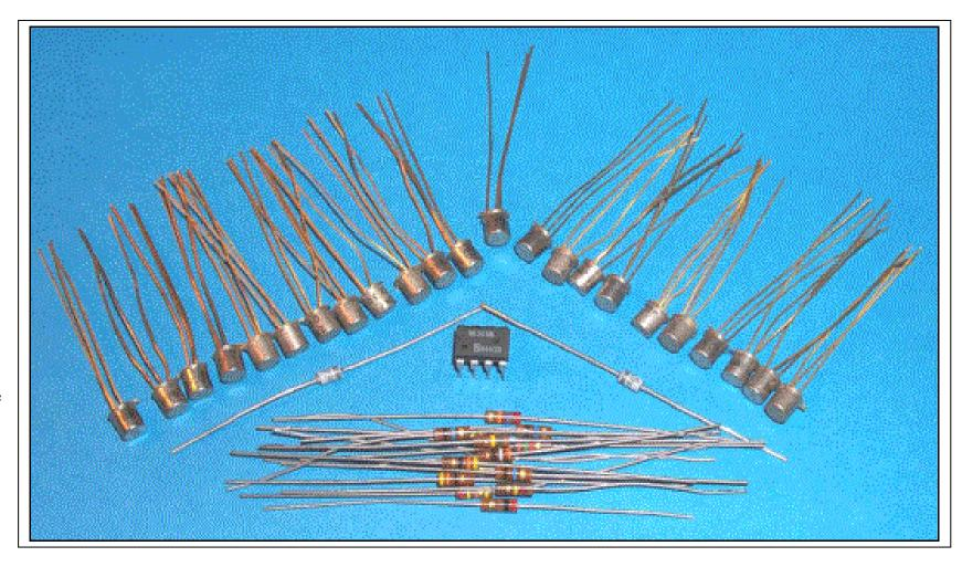
The circuit that is actually inside the "chip" is fairly complex. Here we see the actual complexity of the 555 timer circuit. Hans actually duplicated the circuit with discrete parts before he began the actual chip design and went through about 30 "iterations" or basic design changes before he was happy with the performance of the device.
